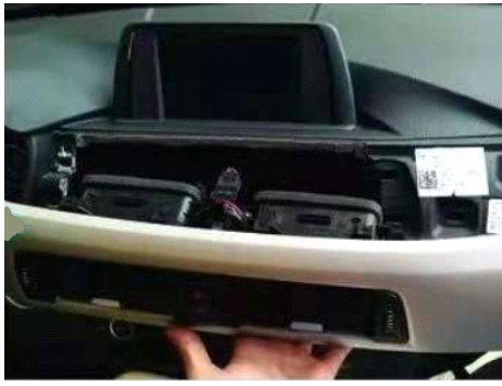
2. Remove AC vent panel.
