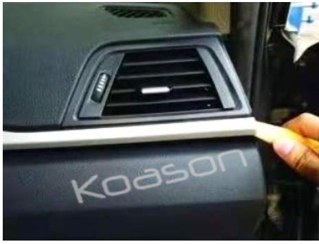
1. Pry up AC vent panel.
