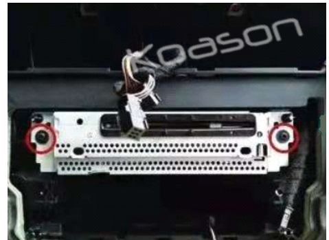
9. Remove screws on CD.
