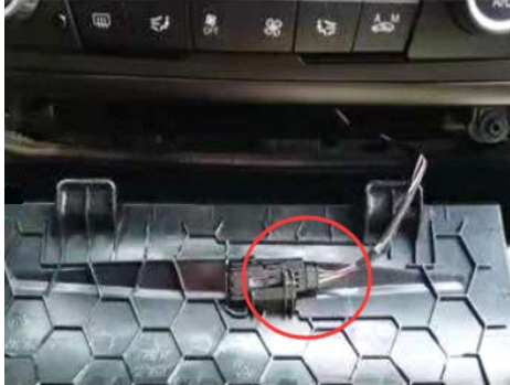
5. Remove flat cable on trim cover.
