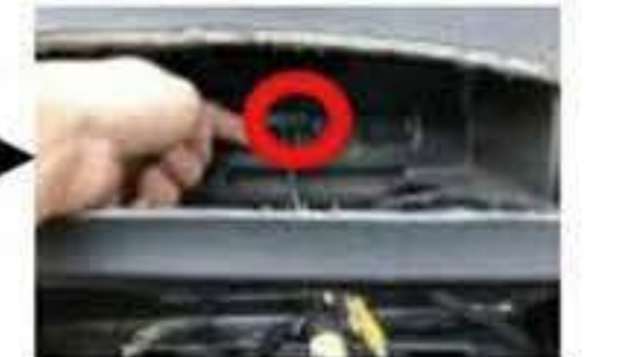
21. Remove the screw in the hole we cut just now.
