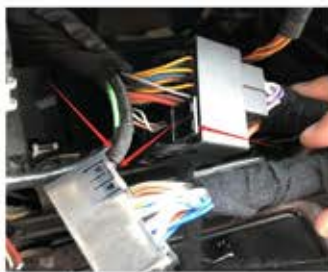
11. Switch fiber cable from original female socket into android male socket
