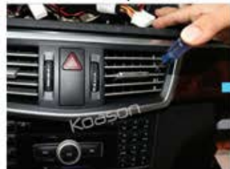
5. Use small slotted screwdriver, move the Air outlet buckle to the middle
