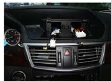
9. Plug LVDS from original monitor to android lvds, NTG4.0 need LVDS switch box
