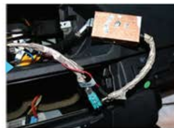
9. Plug LVDS from original monitor to android lvds, NTG4.0 need LVDS switch box
