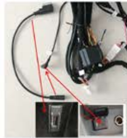
12. NTG5.0: plug USB audio box on power cable to car USB port; NTG4.0/4.5/4.7: plug AUX/AMI into car
