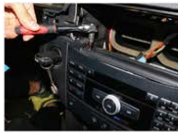
8. Unplug screws on CD, take the CD out little by little
