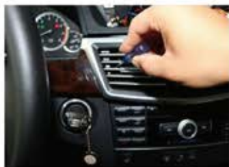
5. Use small slotted screwdriver, move the Air outlet buckle to the middle
