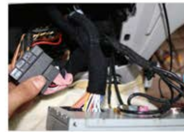
10. Plug android cable to CD
